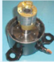
Partially disassembled room air conditioner compressor
